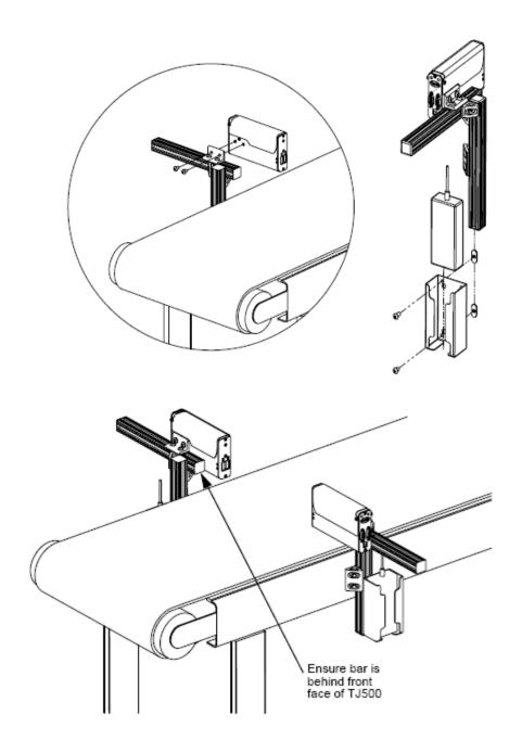
Step 4: Adjust The IP500 Print Head to Substrate
